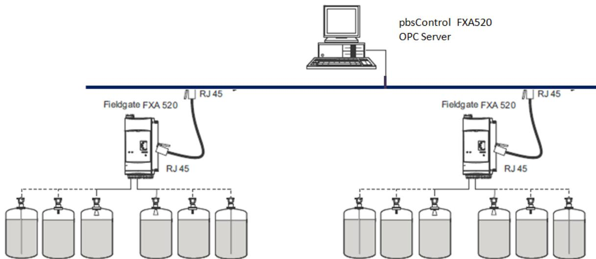
pbsControl FXA520 OPC server is only communicate through Ethernet to FXA520 Gateway .
